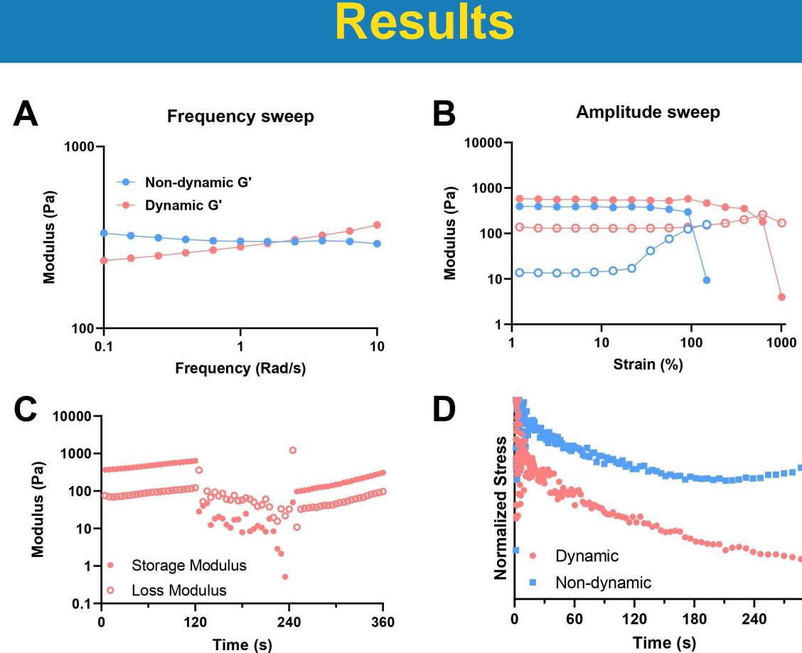
Rheological tests showed that our dynamic hydrogel has superior dynamics. (A) Frequency sweep and (B) amplitude sweep demonstrated that our dynamic hydrogel showed frequency responsiveness and super high fracture shear strain. (C) Step shear test with alternative high (1000%) and low (1%) shear strain exhibited good shear-thinning properties. (D) Stress relaxation test illustrated that our dynamic hydrogel has good matrix remodeling.
